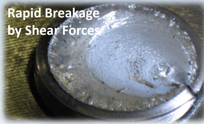
Insufficient Clamp Loads due to Sub-Quality Blind Thread Hole of the Motor Casting Case
