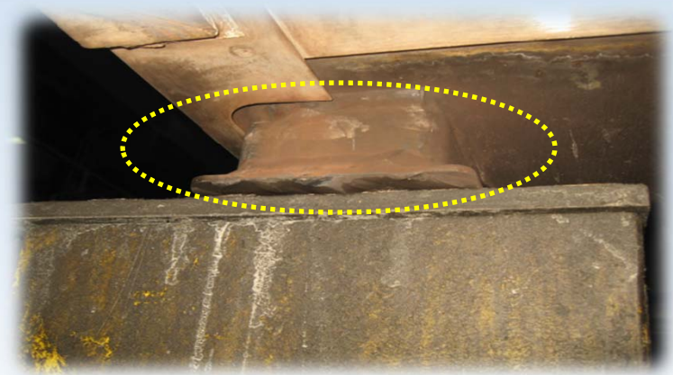
Partial Seating at the Jacking Pad (due to different jacking point locations of older vehicles)
