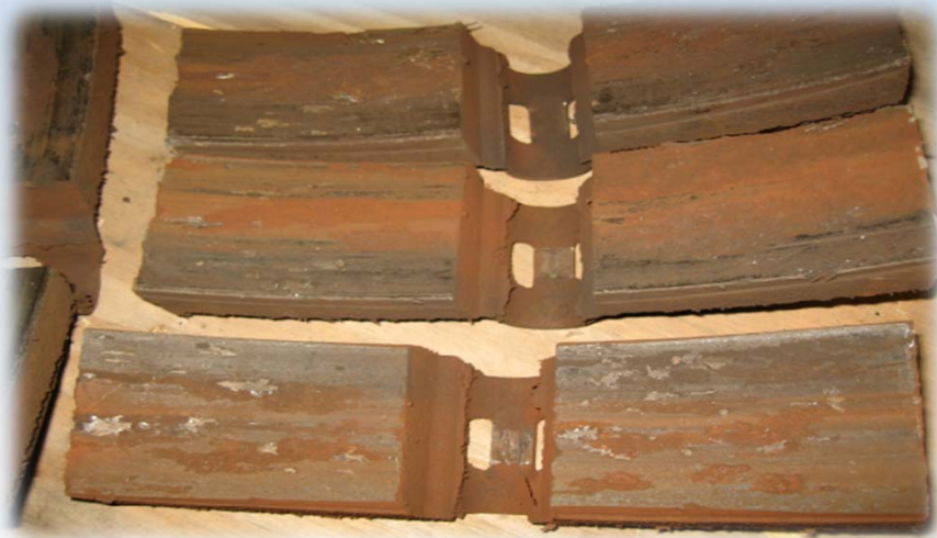
Excessive Grease Picked up by Wheels and Transferred over on Brake Shoes
